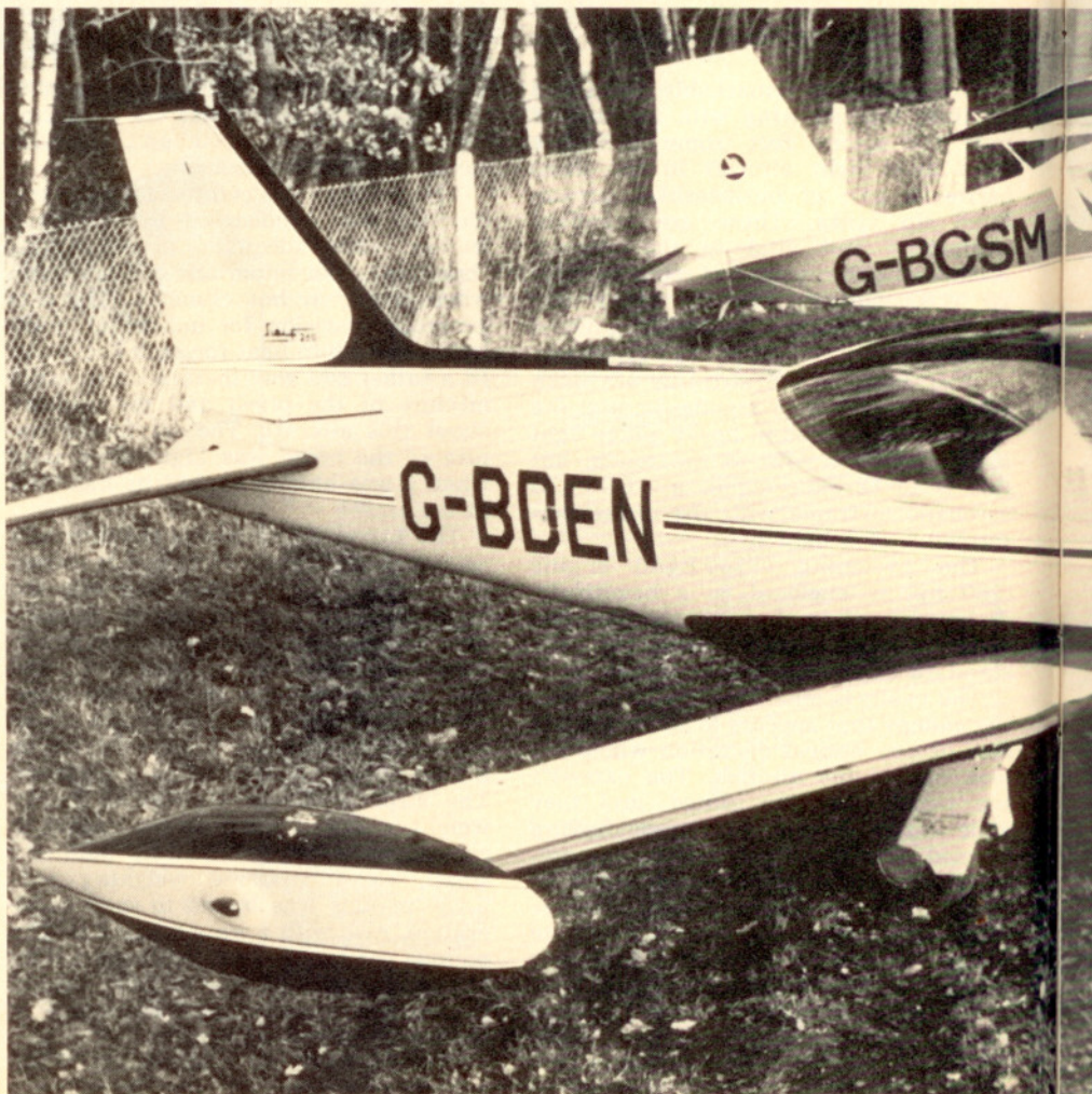
Siai Marchetti F260 is fast (cruise up to 220 mph), economical (up to 17 mpg), aerobatic (+6G -3G) and beautiful to look at. Photo by the author.
